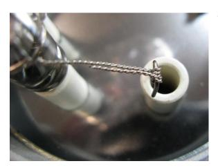
Wrap the ignition wire onto the connecting pin and afterwards onto itself facing the glass body.
